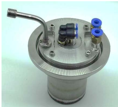
Fig. 1. Photograph of the 2.45 GHz ion source
