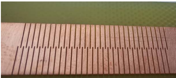
Fig. 1. Photo of the micro-undulator plate with a period of 1 mm used for the electric and mechanical durability tests
