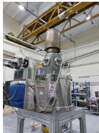
Fig. 1. Photo of a megawatt gyrotron with a frequency of 230 GHz
