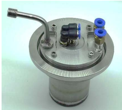
Fig. 1. Photograph of the 2.45 GHz ion source
