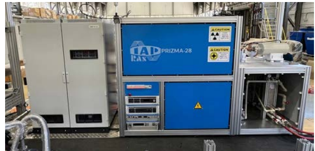
Fig. 2. Photograph of the 28 GHz / 10 kW-based complex for ion sources in JINR
