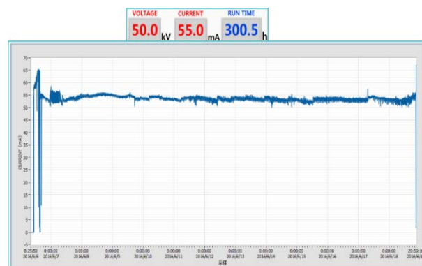
Fig. 2. (color online) Screenshot of the monitor computer at the end of longevity test. Top: extraction voltage, instantaneous current, and counting hours. Bottom: beam current versus elapsed time
